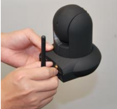
Figure 1.1 Mount the antenna
