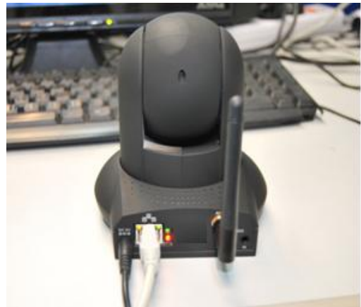
Figure 1.2 Plug the network cable
