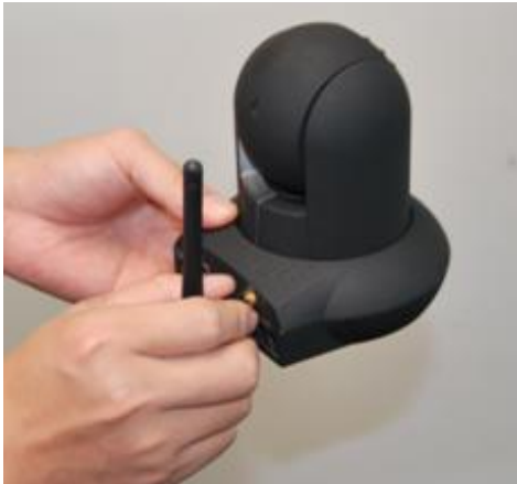
Figure 1.1 Mount the antenna
