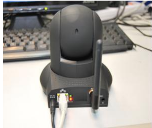
Figure 1.2 Plug the network cable
